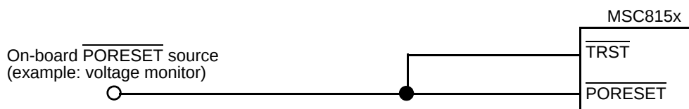
Figure 35. Reset Connection in Functional Application
